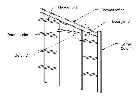
When this is the case, the door jamb will be installed as shown below in Detail C. Note that the top of the door jamb will need to be coped to fit the bottom of the rafter, and the correct sized girt clip that connects the door jamb to the rafter will need to be bent to fit as well. Note that the door jamb base will be installed as shown and described above, as per engineering plans.
